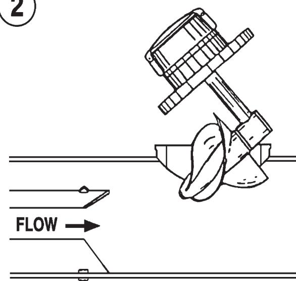
1. Set meter assembly on saddle as shown with one propeller blade pointing down. Propeller should point opposite the direction of flow.
