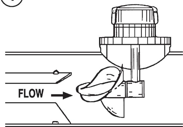
3. Slide the assembly forward and down. The propeller may have to be rotated in order to fit through the saddle opening.
