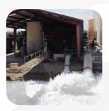
Our large volume test facility is located in Porterville, California. This facility is one of the world's largest volumetric test facilities owned by a meter manufacturer, and it offers accuracy and calibration tests of flow meters from 3 to 72-inch diameter, with flow rates up to 60,000 gpm.
