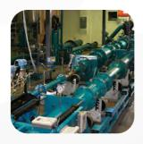
Our Hemet, California factory boasts a robust Calibration Test Lab that enables production of the most accurate and precise flow instrumentation. The test facility utilizes three gravimetric systems and two volumetric systems providing accuracy and calibration tests of flow meters from 1/2 to 20-inch diameter, with flow rates up to 4,000 gpm.
